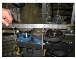
8. Add new chain with an additional  $\frac{1}{2}$  link and connecting link onto the sprocket and sprocket pulley.
