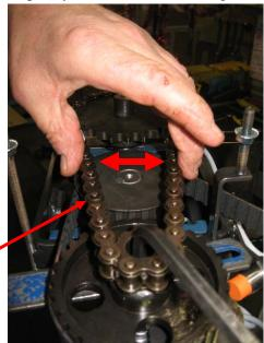
10. Pull outward on the motor end bracket to tighten up the belt and re-tighten motor
