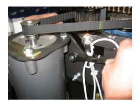
3. Loosen hardware on sprocket pulley.
